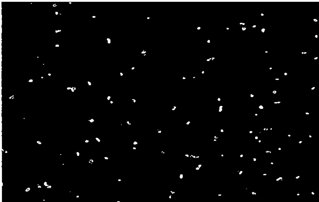
Figure A3-30. Image applying Median filter to remove the noises and small particle other than the bacteria.
