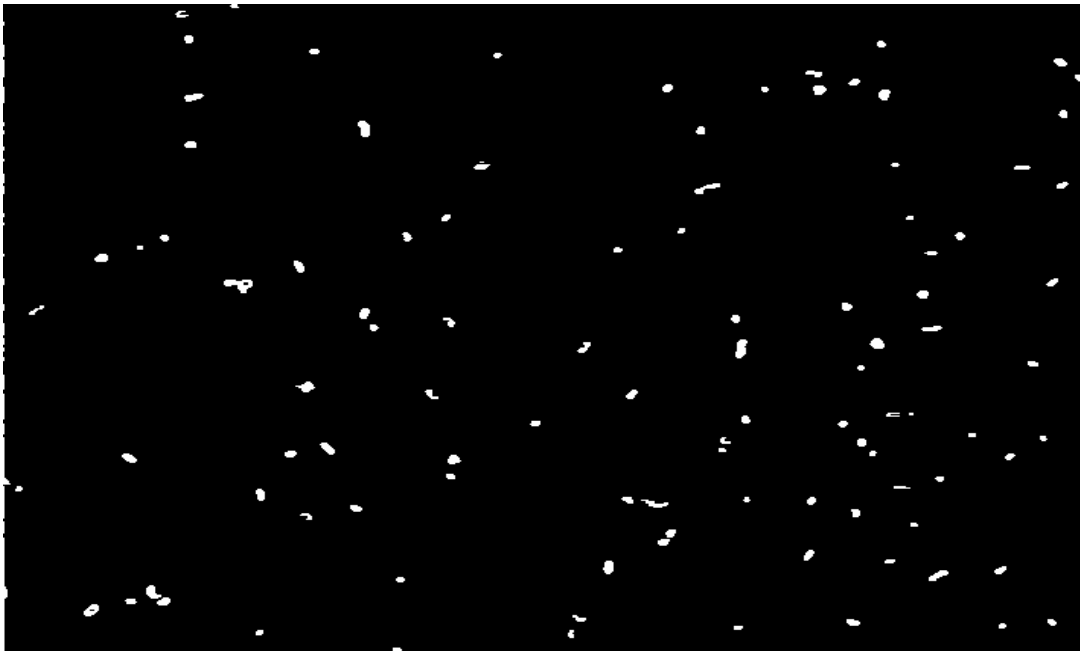
Figure A3-32. Image after the morphological Opening which carefully sharpens the bacteria area.
